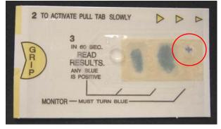
Internal Controls (circled area shown above): **Positive Control: Appearance of Blue Cross Negative Control: White Background behind Blue Cross**
