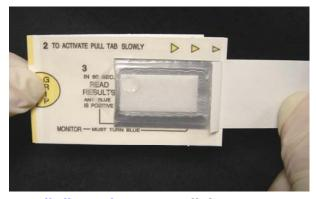
4. Pull silver tab **SLOWLY** all the way to the right and completely remove. Developer pad will "flip over" as tab is pulled.
